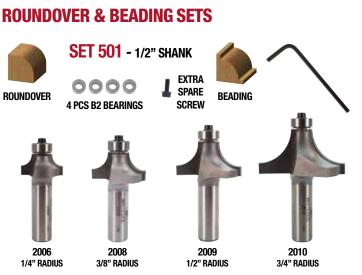
Roundovers are by far the most used edge forming bits in woodworking. This set offers the most common radii (R1/4", R3/8", R1/2") in 1/2" shanks, plus a hefty 3/4" radius workhorse. Extra bearings and wrench are included to convert each bit from Rounding over to Beading - i.e., Roundover with a decorative step.
